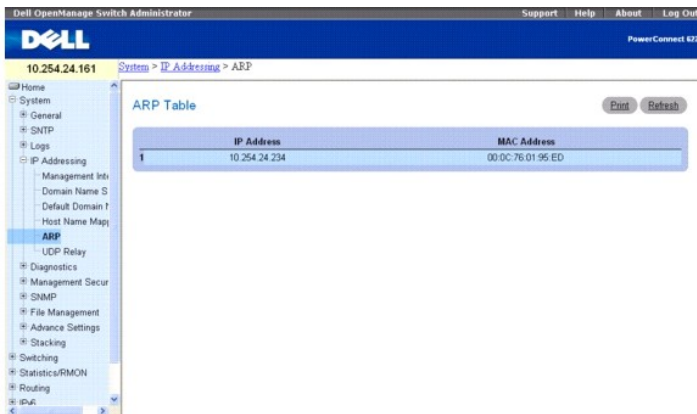
Figure 6-29. Page ARP Table (Table ARP)
