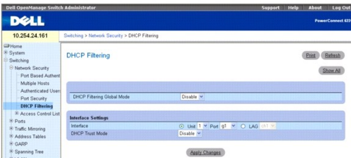
Figure 8-8. Page DHCP Filtering (Filtrage DHCP)
